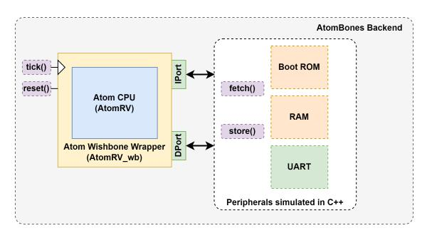
AtomBones backend implements the C++ simulation of SoC peripherals. In each cycle, the backend listens to IPort and DPort for any requests and responds to them by bit-banging. The backend provides the fetch() and store() API that are used to access these memory mapped peripherals.
