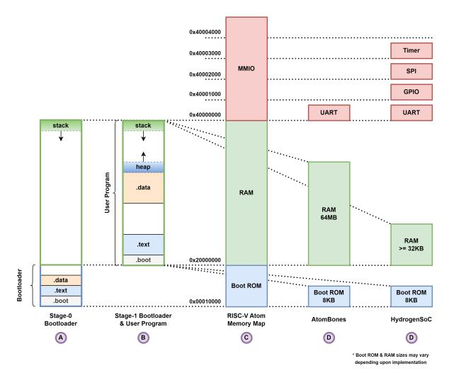
The column  ${\bf C}$  shows the memory map template for all RISC-V Atom based SoCs. Column  ${\bf D}$  and  ${\bf E}$  show the memory map for AtomBones and HydrogenSoC respectively.
