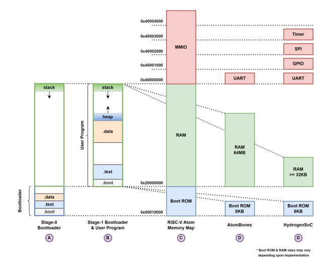
The column C shows the memory map template for all RISC-V Atom based SoCs. Column D and E show the memory map for AtomBones and HydrogenSoC respectively.
